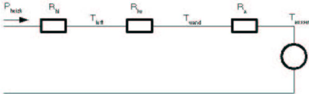
In this state of equilibrium the temperature differential between room air ( $T_{\text{luft}} = 36^\circ\text{C}$ ) and outside temperature ( $T_{\text{ausssen}} = 11^\circ\text{C}$ ) drops only at the series circuit of the surface heat transfer resistance air/wall  $R_{\text{lw}}$  and the loss resistance to the exterior  $R_a$ . It follows that:
