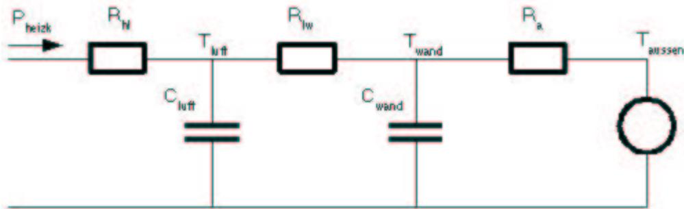
The heating power  $P_{\text{heizk}}$  warms the air mass  $C_{\text{luft}}$  through the surface heat transfer resistance heater/air  $R_{\text{hl}}$ . It continues to flow over the surface heat transfer resistance air/wall  $R_{\text{lw}}$  into the wall capacity  $C_{\text{wand}}$  (the material mass of the wall) and over the insulation resistance  $R_{\text{a}}$  to the exterior, whose temperature is assumed to be constant at  $T_{\text{aussen}}$ .
